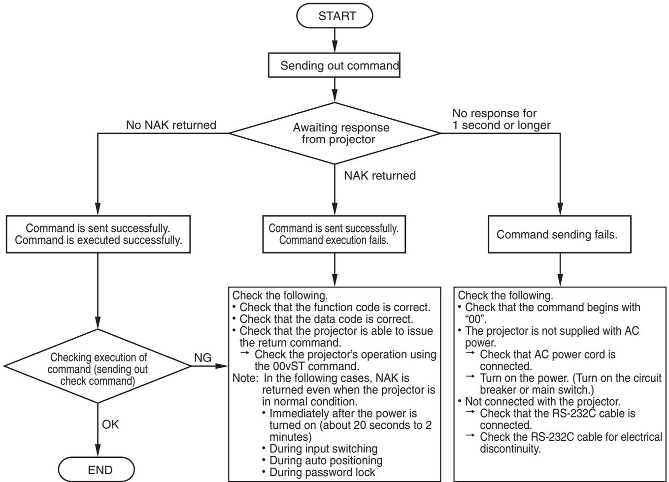
**[Method of checking state of projector]**
