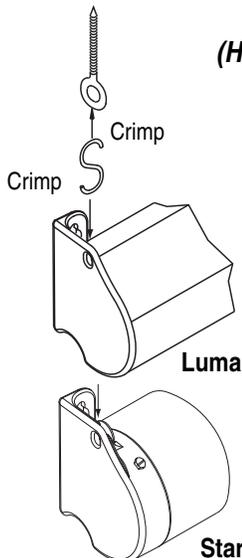
Use the holes at the front of the endcap/mounting bracket for suspended mounting. Position and properly anchor screw eyes or other fasteners (not included) into ceiling joists or other solid surface. Suspend "S" hooks (not included) from fasteners (not included) and hook through holes in the front of the mounting bracket. For added safety, crimp both ends of the "S" hooks so the screen cannot come off.
