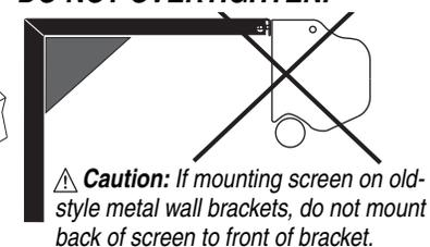
**⚠ Caution: If mounting screen on old-style metal wall brackets, do not mount back of screen to front of bracket.**
