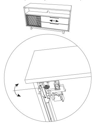
Lateral Adjustment: Turn White Wheel on both mechanisms to adjust drawer position left or right.
