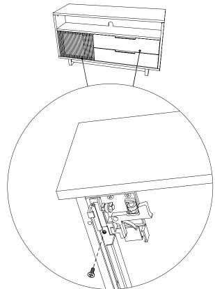
Two (2) adjustment mechanisms are found on underside of each Vertica drawer, at left and at right. **All drawer position adjustments require removal of indicated screw on both adjustment mechanisms.** Save screws for re-installation prior to any future cabinet shipment.
