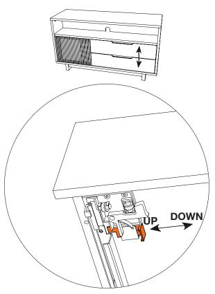
Vertical Adjustment: Manipulate Orange Lever on one or both mechanisms, as necessary, to adjust drawer position up or down.
