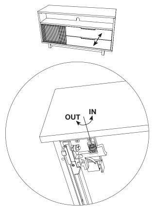
Front-to-Back Adjustment: Turn Black Wheel on one or both mechanisms, as necessary, to adjust drawer position in or out.
