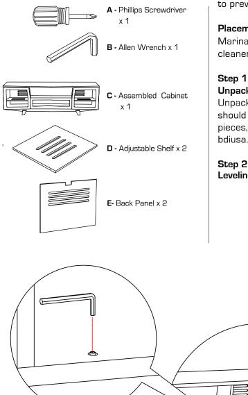
The adjustable leveler glides on the bottom, mid section of the cabinet are accessible from inside the cabinet using the Allen Wrench (B).
