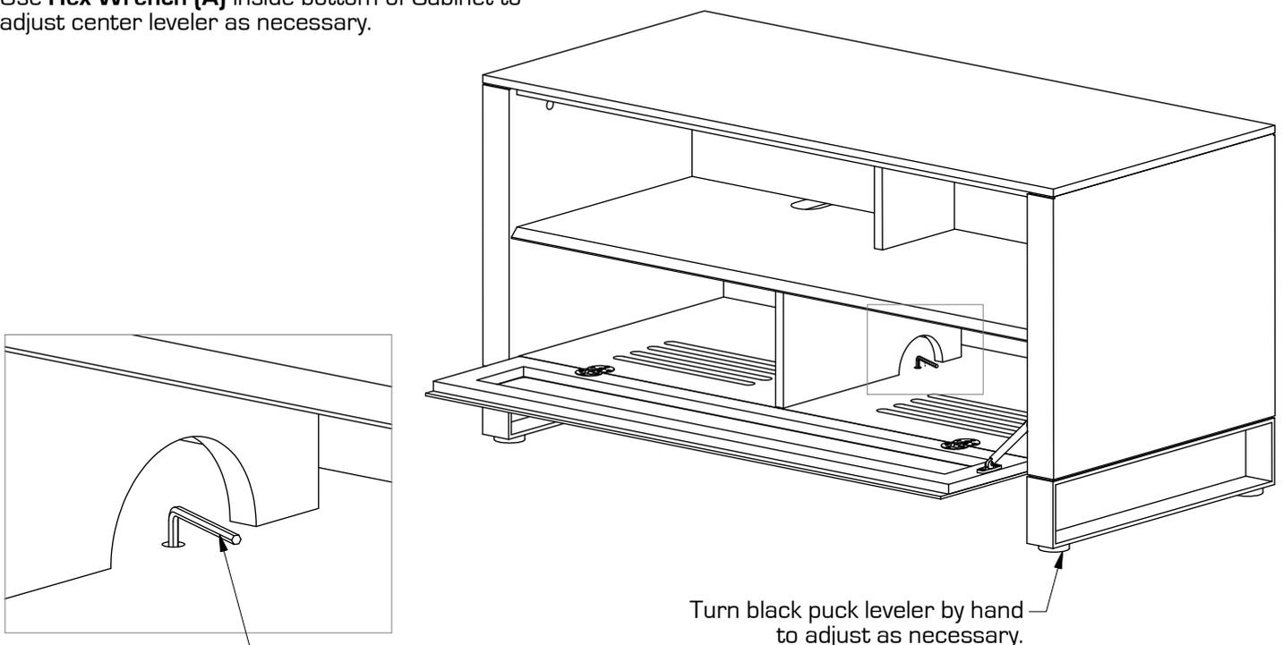
Use **Hex Wrench (A)** inside bottom of Cabinet to adjust Leveler as necessary.
