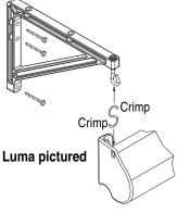
Wall mount the brackets (not included with screen) using hardware recommended for "Wall Mounting" (above, not included). Then, suspend the screen from the front holes with "S" hooks. For added safety, crimp both ends of the "S" hooks so the screen cannot come off.
