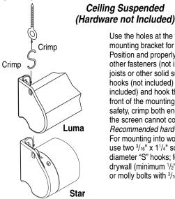
Use the holes at the front of the endcap/ mounting bracket for suspended mounting. Position and properly anchor screw eyes or other fasteners (not included) into ceiling joists or other solid surface. Suspend "S" hooks (not included) from fasteners (not included) and hook through holes in the front of the mounting bracket. For added safety, crimp both ends of the "S" hooks so the screen cannot come off.
